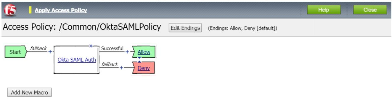
An access policy consists of a start point, actions, and one or more endings. To insert a new action, click on the + sign. To configure an action or ending, click on the link inside the box. To delete an action, click on the x on the upper right edge of the box. Click the **Add Macro** button to add a purpose-built set of predefined access policy items, to simplify access policy creation.
